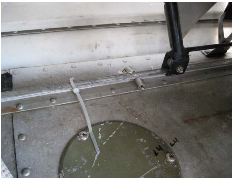
Cessna 182 with cotter pin and spacers installed for pilot Seat, aft seat stop (The tie wrap was “extra”).
