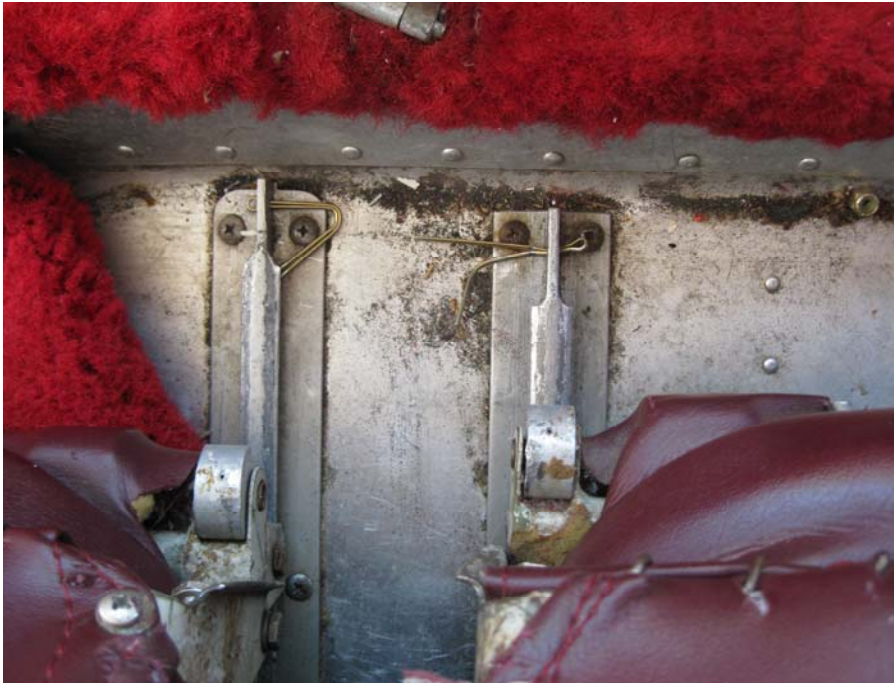
Cessna 150 with cotter pins “installed” for aft seat stops.
